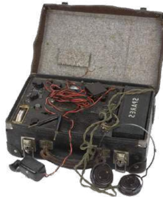
© IWM COM 229 stereo transmitter and receiver radio set, set within a miniature suitcase for use by British SOE and intelligence agents during the Second World War
